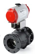
PEEK seats offer high pressure/temperature capability. Tek-Fil® seats offer reduced torque in high temperature, high cycle, and steam service applications. TFM 1600 seats offer the exceptional chemical resistance of PTFE plus lower porosity and permeability, improved temperature range and reduced valve torques.
